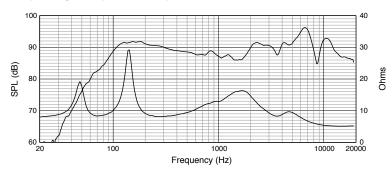
Frequency response in half-space (2pi, mounted in ceiling, 1W, 1m), impedance at  $8\Omega$  (low-impedance) setting
