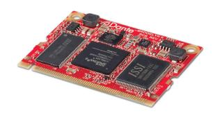
In combination with Audinates virtual soundcard and Televic's TReX software a PC can be turned into a multichannel recording station, just by connecting the network port of this PC to the network. Very cost effective as no audio interfacing equipment is required.
